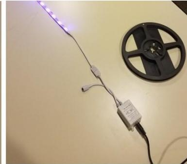
RGB control box connected to light strip
