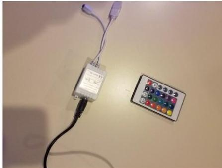
Power supply connected to RGB control box
