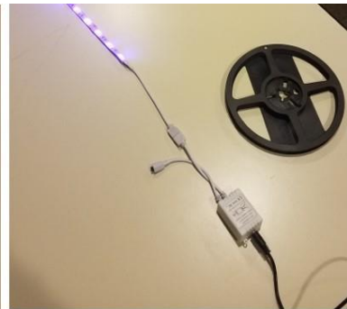
RGB control box connected to light strip
