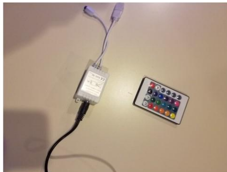
Power supply connected to RGB control box
